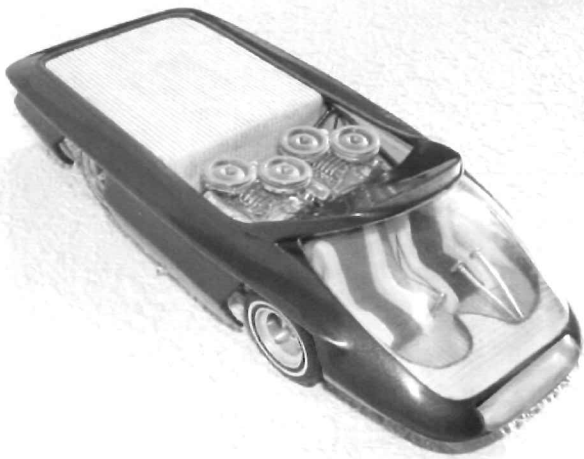
Another wild custom contest winner from the early '60s is Robert Sifferd's "Telstar." It features a dual mid-engine drive-train and a unique bubble-enclosed cab. It is being cloned right now by Mitch Capps.
