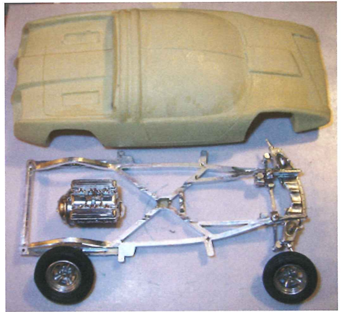
Here is the relative relationship of the parts. This will be a great model when finished!
