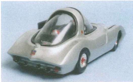
The rear of the car was as stunning as the front clip. The center-mounted exhaust are angled upward, ala Jag XKE.
